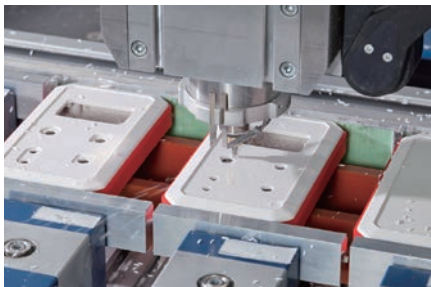
7. Machining on enclosure
