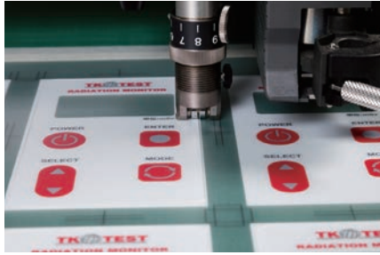
5. Cutting the sheet to size
